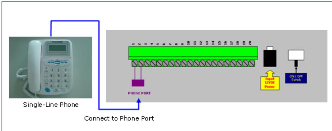
**Note:** Before commencing programming it is advisable to read the below programming setting instructions thoroughly. To start with programming, user must plug-in a normal single line phone to TEL1 (Port 1)
