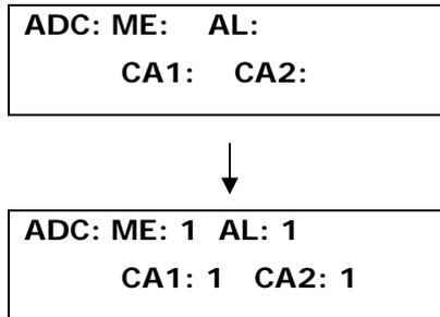
**Example:** Setting the unit to generate an Alert Message, call the administrators, generate a pulse (+5V) and sound the audible alarm when AC failed.
