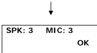
*Note:* Both SPK and MIC volume level range from 1 – 4 (**Default:** 1). Adjust the speaker and microphone volume to compatible with your alarm panel
