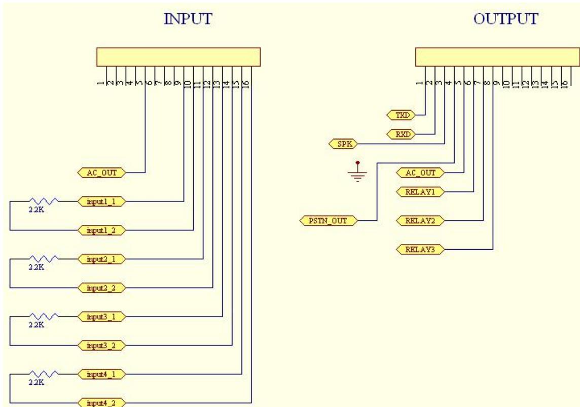
A 2.2K Resistor must be attached along with the sensors for all inputs
