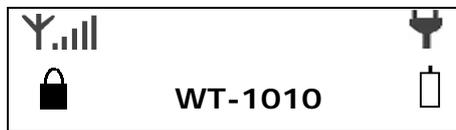
When the system is in Disarmed Mode, an unlock icon will be displayed as shown below
