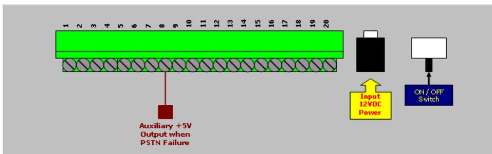
**Note:** PSTN Failure Output facility can be used on alarm panel for alert notification
