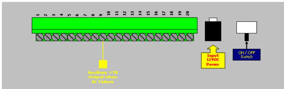
**Note:** Power Down Output facility can be used on alarm panel for alert notification
