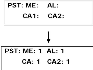
**Example:** Setting the unit to generate an Alert Message, call the administrators, generate a pulse (+V) and sound the audible alarm when PSTN failed.
